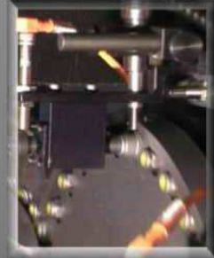
Cracks detection by Eddy Current probe and piece's rotation control
