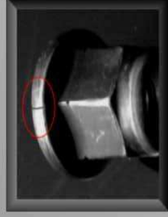
Cracks detection by Eddy Current probe and piece's rotation control
