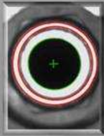
CAMERA 1: Nylon washer integrity and closure, Clinching control
